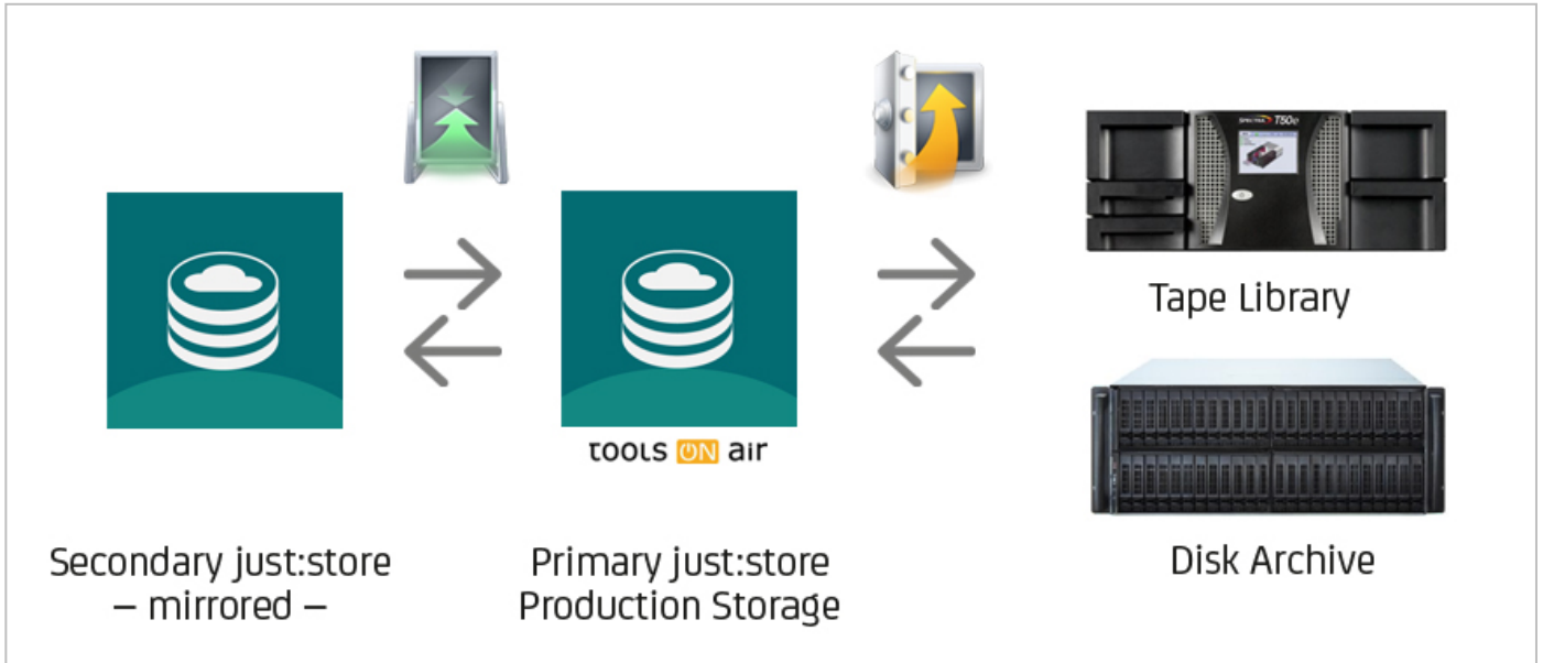
Full just:store and Archiware P5 production setup: P5 Synchronize for data Cloning, P5 Archive for long-term Archiving
